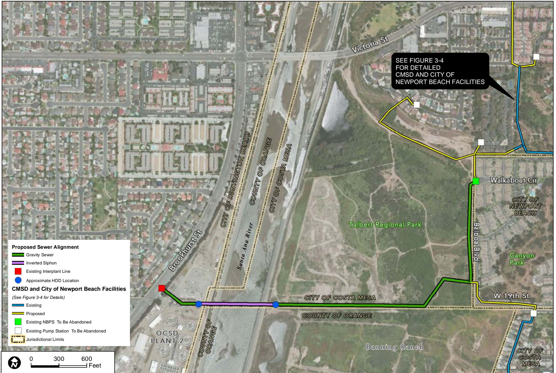
FIGURE 3-3 Proposed OCSD Southwest Costa Mesa Trunk Sewer Project No. 6-19 Alignment
