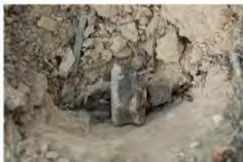
Photograph 4: Asphaltic material excavated from shallow pit
