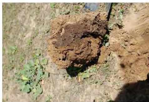
Photograph 5: 2.5 inch thick layer of Asphaltic material in C Extended 3.
